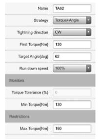
The tolerance for OK is +- 3 degrees
